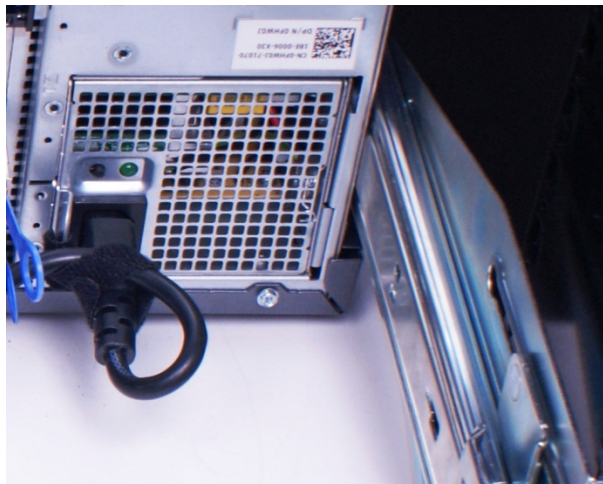
Figure 3. Routing the power cable through the strain relief on a fixed power supply
